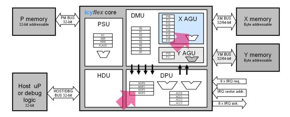
DSP-type features: zero-overhead hardware loop, complex addressing modes, high and balanced throughput
