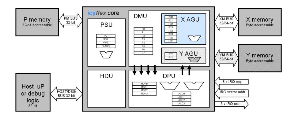
3 separate busses  $\rightarrow$  up to 3 parallel accesses every clock cycle less clock cycles  $\rightarrow$  less power consumption
