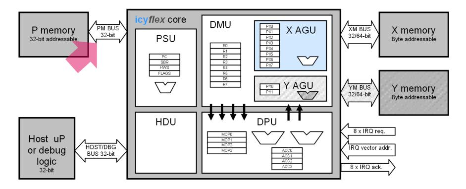
customizable at synthesis  $\rightarrow$  busses can be shrunk, blocks can be removed only useful logic is integrated  $\rightarrow$  less power consumption
